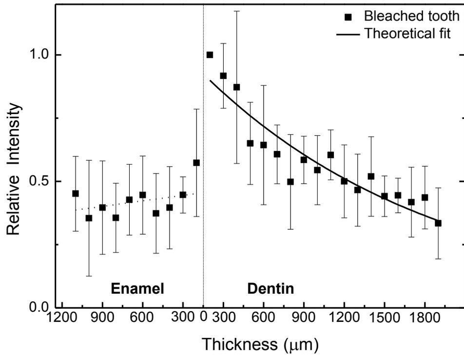
3) Relative intensity of the O-O stretching band as a function of specimen's depth. Lateral analysis demonstrating that  $H_2O_2$  crossed the enamel layer, had increased concentration at DEJ, and accumulated in the dentin.
