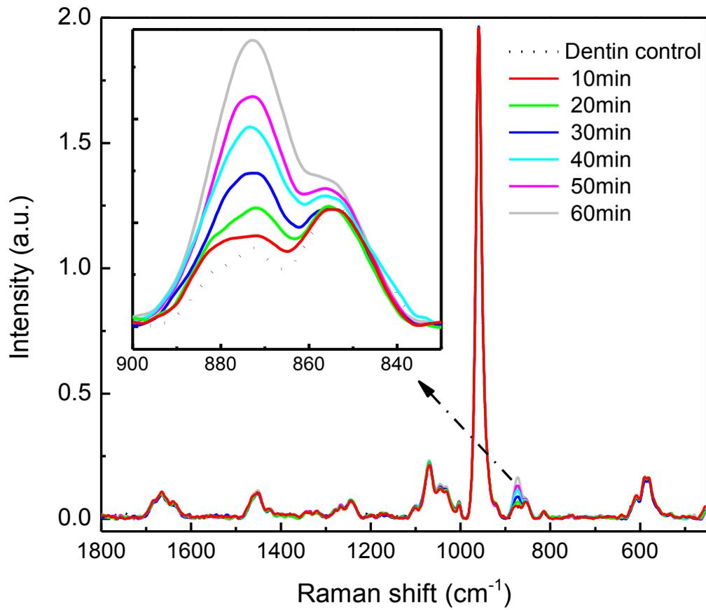
2) Raman spectra of dentin with and without treatment monitored over 60 minutes (DS2). Raman spectrum shift at around 873cm<sup>-1</sup> is attributed to the stretching O-O. Raman band growth started at 10min for the treated group and continued rising for up to 60min.
